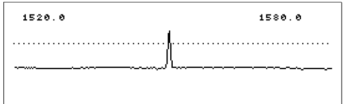
PRBS modulation graph showing raised noise floor.
