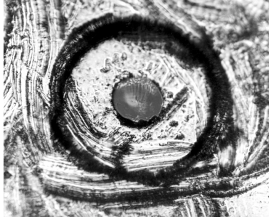
Figure 8-6. Damage from improper cleaning.
